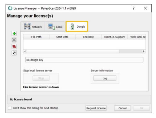
• If the dongle key has not been inserted yet, plug it. The dongle key ID must be displayed. If not, please check the <u>chapter D. Common issues</u>.
